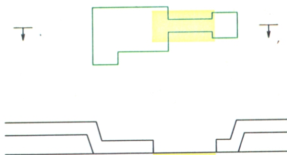
Fig.10. Patterning Ion Implantation
