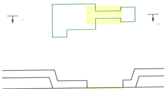
Fig.10. Patterning Ion Implantation
