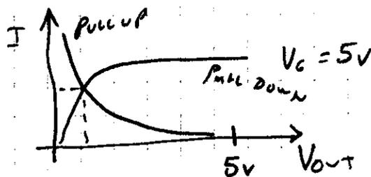
So: Low drive as try to bring  $V_O$  back up and high current needed to bring  $V_O$  down.
