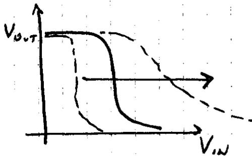
arrow shows effect of decreasing the relative "length" of the load T with respect to the inverter T.
