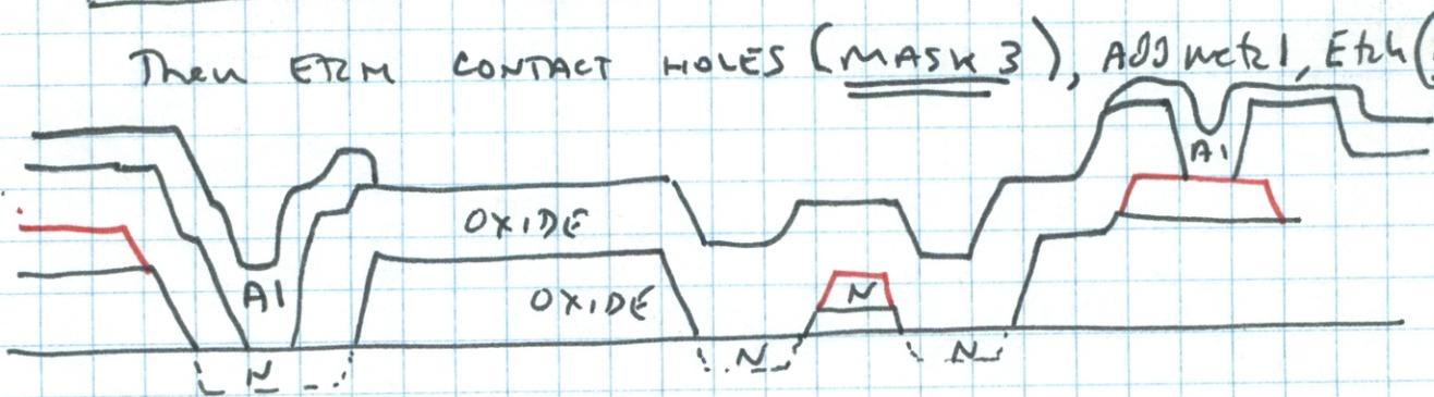
NOTE: BRING GATE CONTACTS UP TO POLY ON TOP OF THICK OXIDE LAYER, TO PREVENT PROBLEMS OF SOLUTION OF GATE SILICON INTO AL.
