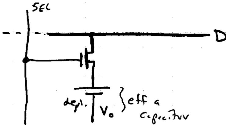
TO WRITE: Put D on, hit select. Charges C to 1 if D=1. Disch. to 0 if D=0. Row unselect. Slow leakage to substrate. Refresh in ~ 1ms.
