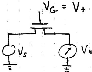
The threshold is a function of  $V_S$  because of effect of substrate:
