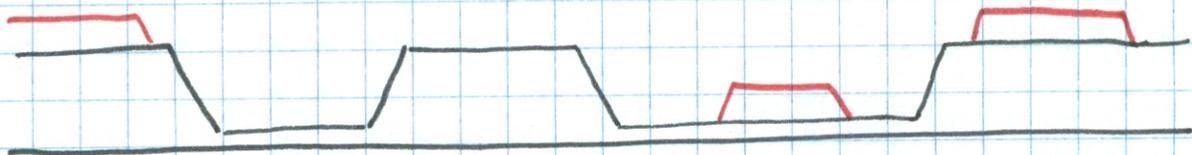
AFTER ETCH OXIDE: THEN IMPLANT Phosphorus IONS to form N-Type Regions
