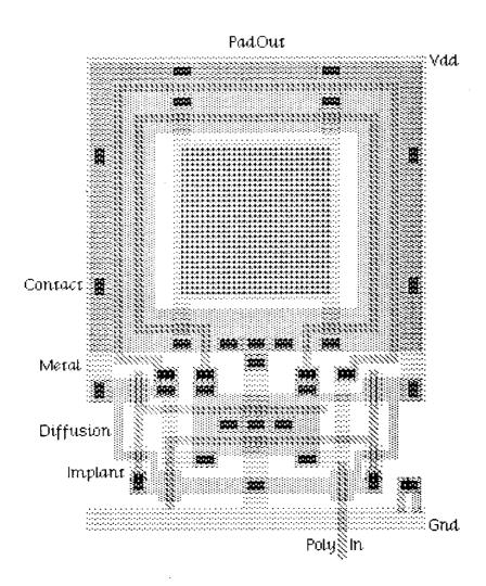
Figure 2.4.1. Icarus Layout of "PadOut"
