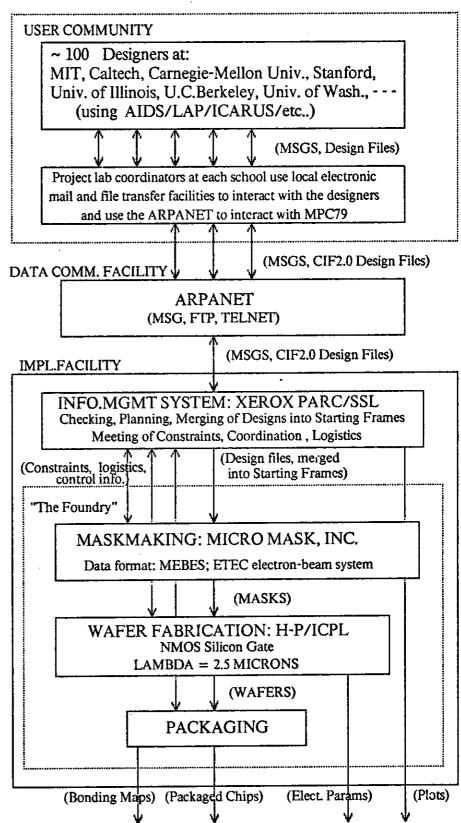
Packaged Chips, custom wire-bonded per project, along with plots, wire-bonding maps, and results of electrical testing, to send back to the designers for functional testing.
