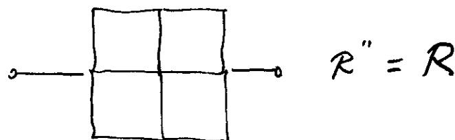
So, for given thickness, Resistance is same for  $\square$  of any size.
