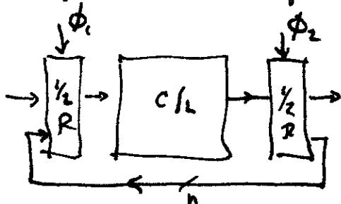
Some of the outputs are fed back around to the input register.
