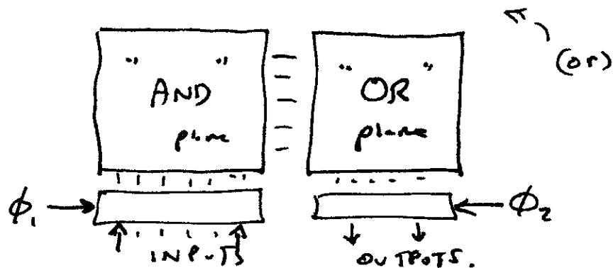
An EXAMPLE CIRCUIT: TO ILLUSTRATE Fcn OF THE AND & OR Planes. THEY ARE REALLY NOR planes, but as you know NOR-NOR logic (if inputs = 1 available True & Comp form can generate all C/L functions of the inputs), just as AND-OR logic can.
