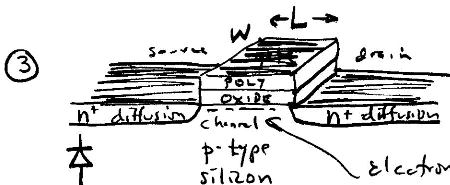
Electrons attracted if  $V_{gs} = V_{th}$
