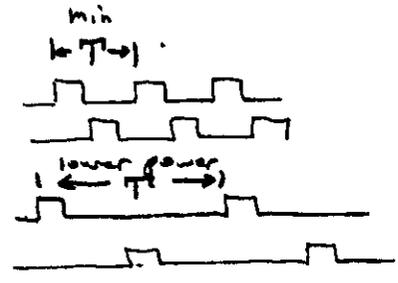
NO STATIC PWR DISS WHEN CLOCKS OFF! IF LOW DUTY CYCLE, THEN LOW POWER (BUT LONG T compared to min T)
