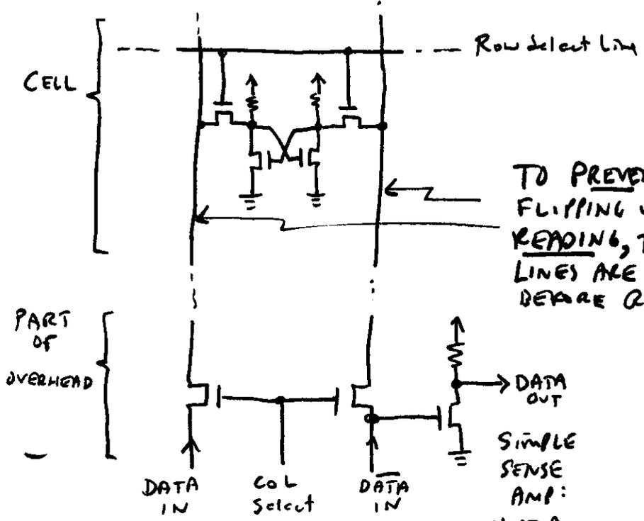
TO PREVENT FLIPPING WHILE READING, THESE LINES ARE PRECHARGED BEFORE READING
