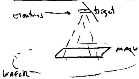
If use traditional method of producing soft X-rays, have problem of not a "point source" and beam is not collimated. So, if put close to source to get higher intensity, resolution is poor. If further away, exposure takes too long.
