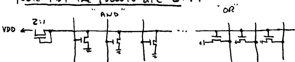
It was designed so that the PULLDOWNS could be 1:2. This makes the ratio 4:1 as required. BUT NOTE, if you programmed it with min width diffusion lines, you would make pulldowns that were 1:1, and overall ratio would be only 2:1.
