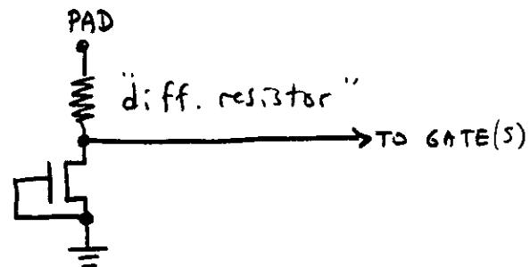
But, if Voltage becomes large (i.e. Pad struck by lightning) then FET will punch through, current will flow dropping the overvoltage across the resistor.
