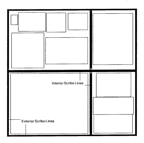
Figure 4.2. Overall View of a Multi-Project Chip
