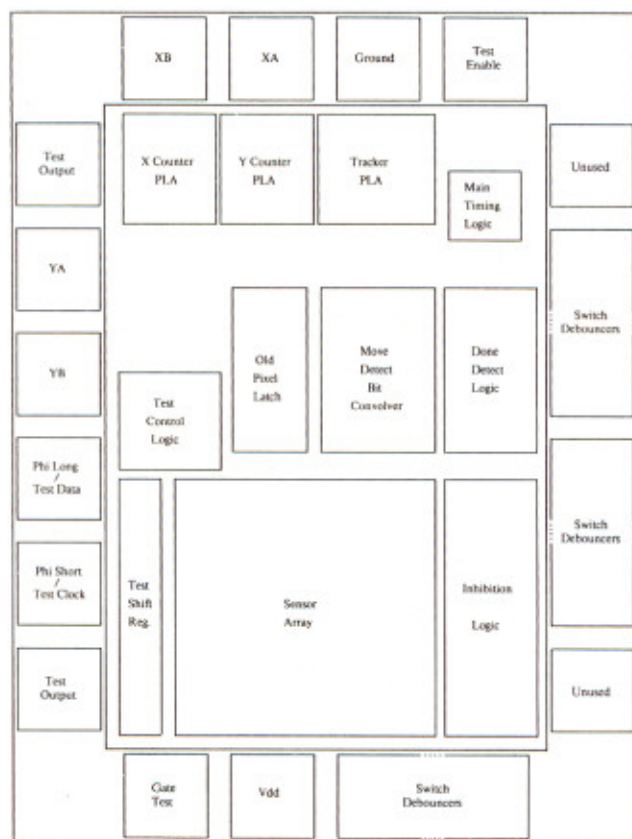
FIGURE 11. a) Photo of the improved optical mouse chip. b) Floorplan of the improved optical mouse chip.
