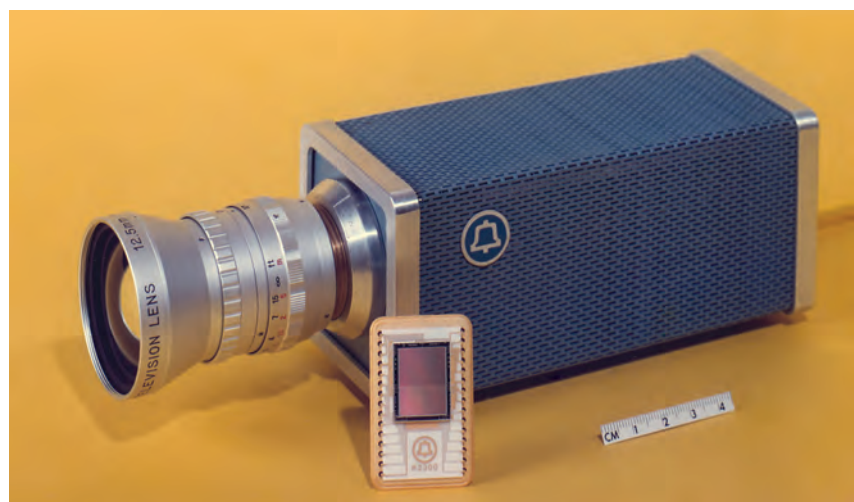
FIGURE 1: The first solid-state image sensor compatible with the American broadcast TV format.
