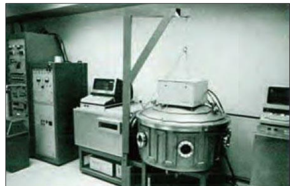
FIGURE 3: Computer-controlled plasma system at HP’s ICPL. (Courtesy of Hewlett-Packard [12])
