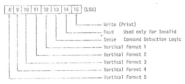
3.3.3.2.2 Each of the <u>Vertical Format</u> Control Codes required for these line printers is one less, in binary value, than the corresponding codes used in standard software. The vertical format bits from the command register outputs are applied to VF code decrement logic which decrements the binary value, thus correcting this discrepancy. The outpus of this logic are available to the LP Data Multiplexor.
